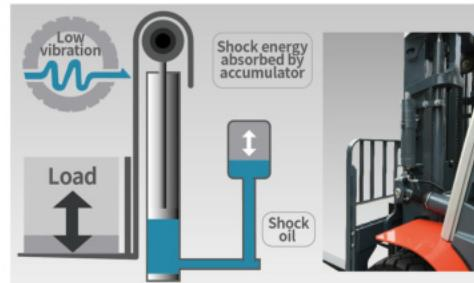
Standard configuration of oil cylinder lower buffer, comfortable operation
