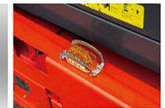
Emergency falling and dual flashing warning lights
