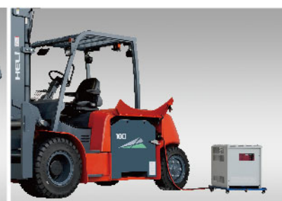
Interlocking vehicle fast charging interface
